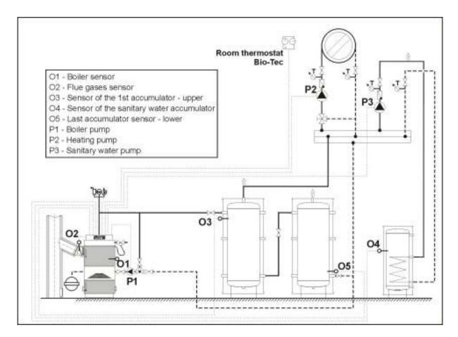
Figure 3. Scheme of the system – connecting points for sensor and pumps
