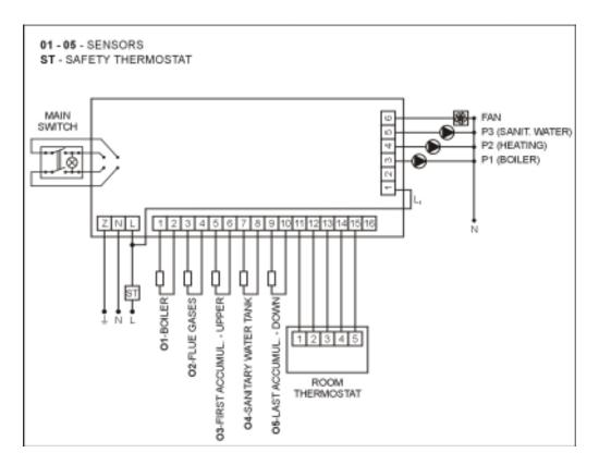
Figure 2. Electrical scheme for the regulator connection
