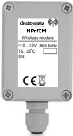
The HPPrFCM radio module is standard equipment for the thermostat.
