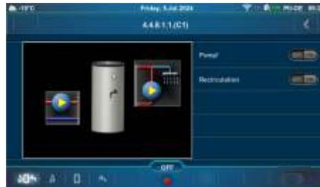
It is necessary to press the "ON" button next to the symbol of the pump/valve for which you want to check whether it is running. The pump symbol will start to rotate and button will light up green. After pressing the "OFF" button, the pump will stop operating.
