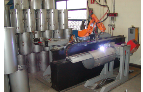
Robotic welding of stainless steel water heaters
