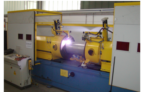
Automated welding of stainless steel water heaters
