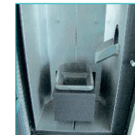
Burning chamber grate
