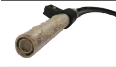
Dirty photocell which can result error in ignition or flame dissapear error
