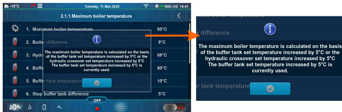
d) If is selected **And another heating controller** (menu Installation -> Configuring -> Boiler control: And another heating controller)
