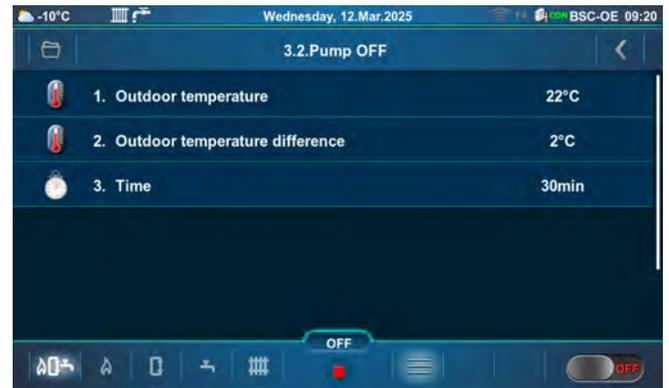
Configuration: 1, 2, 3, 4, 5, 6, 7, 14, 15, 18, 19, 21, 22, 23, 24, 25, 26, 27, 28, 29, 30, 31, 32, 33, 34, 35, 36, 37, 38, 39, 40, 41, 42 - if the measured outdoor temperature is higher than the set outdoor temperature + set outdoor temperature difference for the duration of the set time the heating circuit pump is turned off.
