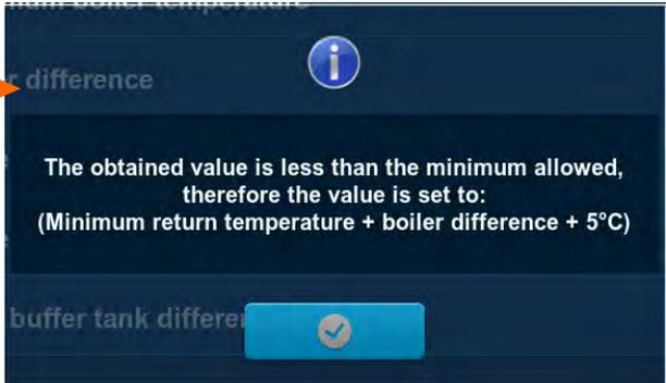
2b. Buffer tank temperature set to < DHW set temperature
