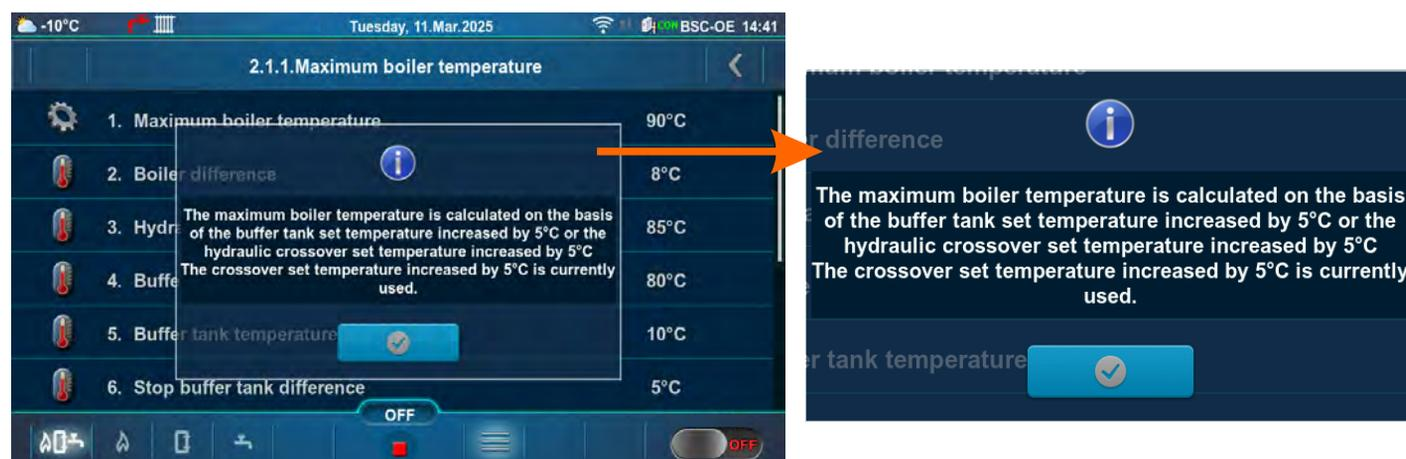
2. Hydraulic crossover temperature < Buffer tank temperature
