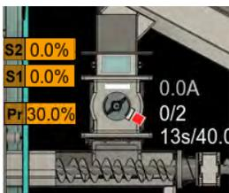
This procedure repeats in a cycle (loop), and it is controlled by the boiler controller. On the side of the rotary valve, there are two inductive sensors (6) that provide information to the boiler controller on whether the rotary valve chambers are open or closed.
