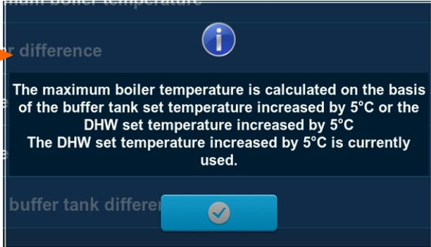
2. Buffer tank temperature set to <65 °C:
