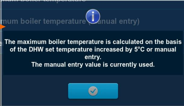
2. (Temperature DHW + 5 °C) > Maximum boiler temperature (manual entry):
