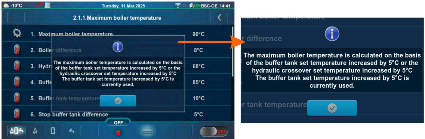
b) If is selected **Only boiler regulation** (menu Installation -> Configuring -> Boiler control: Only boiler regulation) and if as Temperature maintenance is selected **Boiler** (menu Installation-> Configuring -> Temperature maintenance: Boiler)
