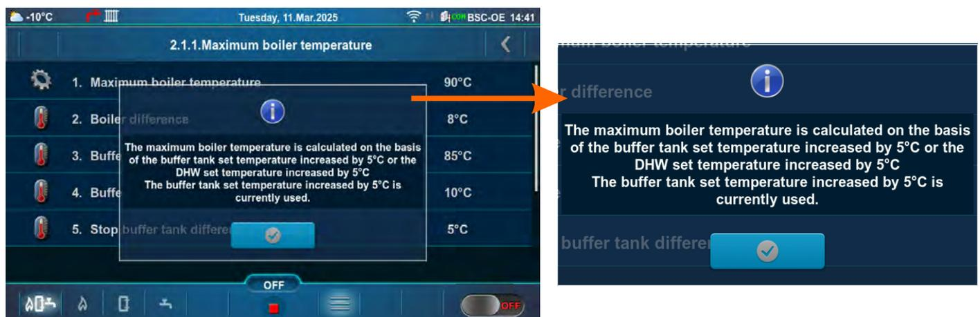
1b. Buffer tank temperature set to < DHW set temperature
