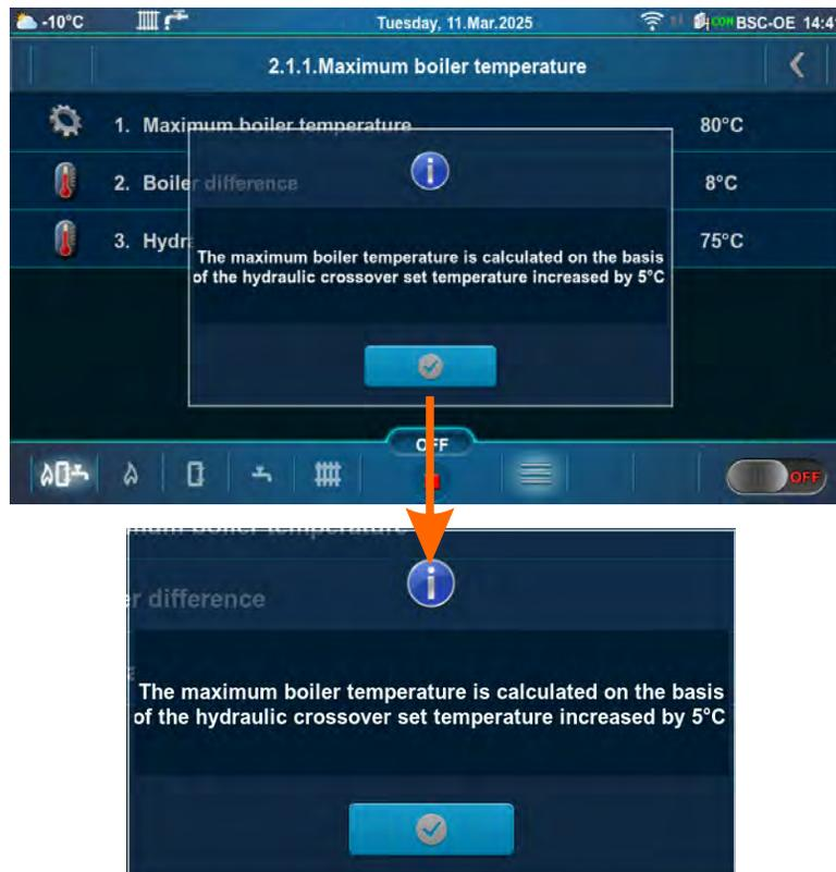
d) If is selected **And another heating controller** (menu Installation -> Configuring -> Boiler control: And another heating controller)
