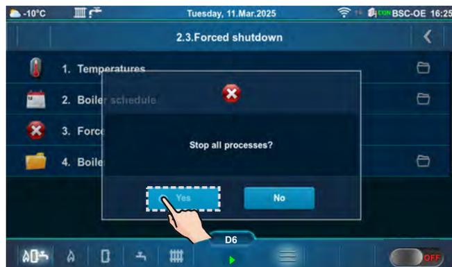
**IMPORTANT!** To be able to stop all processes, you must first switch off the boiler in the usual way by switching ON
