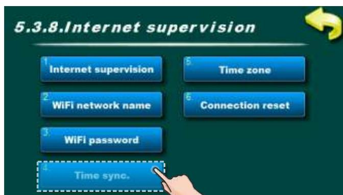
This option allows boiler time synchronization with web server time (internet time).
