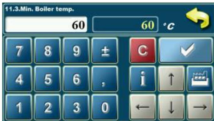
Adjustment of minimal boiler temperature when is chimney sweeper mod activated.
