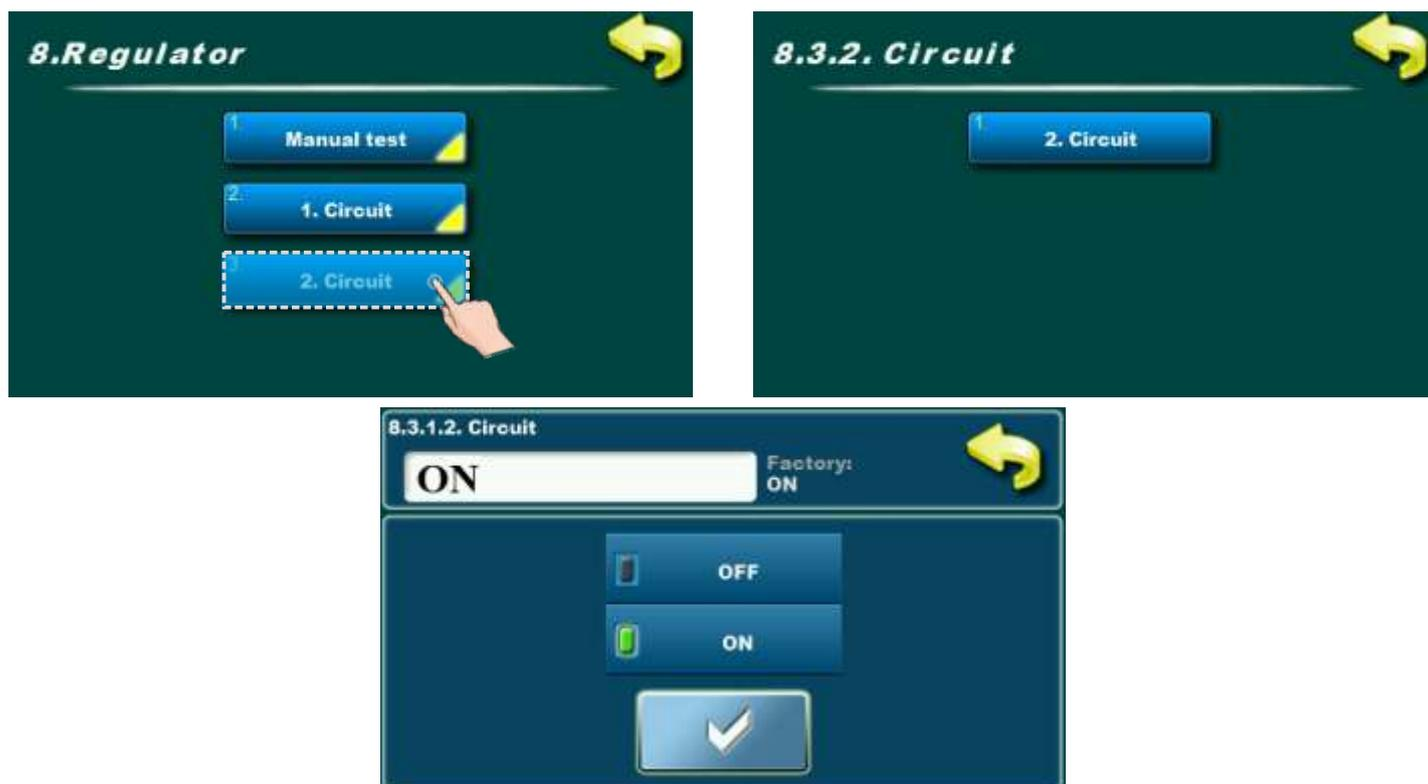
Option for turning on / off second heating circuit.
