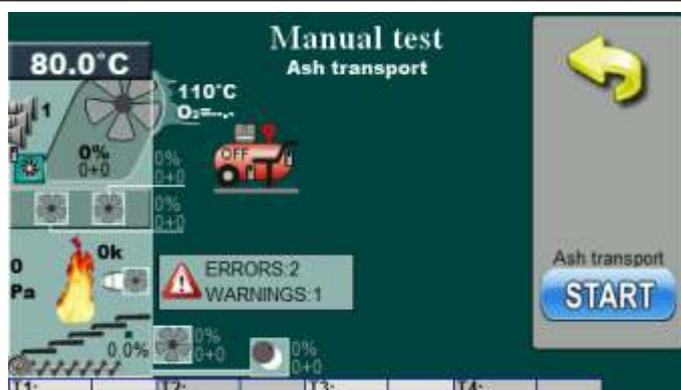
Option for Ash transport test. By pressing „START” button Ash transport will be start with work.
