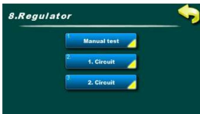
Menu „Regulator” is showed only if module for two heating circuits CM2K is installed and configured.
