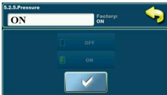
Option for pressure switch turning on/off. It is not possible to change this parameter.
