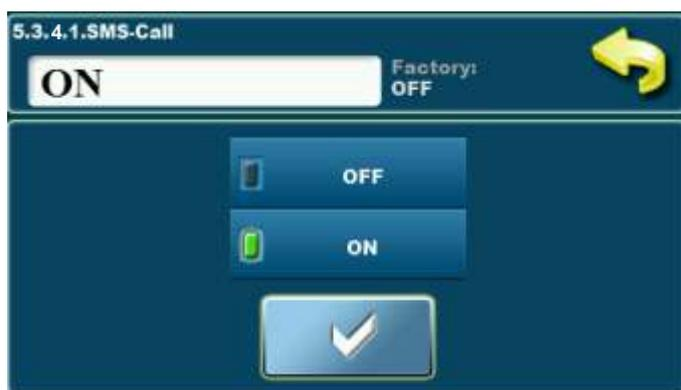
Option for turning ON/OFF sms-call (if is installed and configured GSM module).
