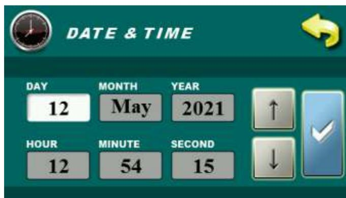
This option is used to set the date and time. It is necessary for starting times, and the recording of errors / warnings (for the occurrence of errors / warnings, remembers the date and time of occurrence). After setting the date and time it is necessary to press the "CONFIRM" for saving date and time. The clock could be faster/slower (the shift could be 2-3 minutes per month), which is considered normal and we recommend that you adjust it periodically.
