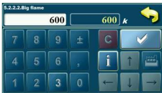
Value of photocell resistance in which will be control unit register big flame in boiler. It is not possible to change this parameter.
