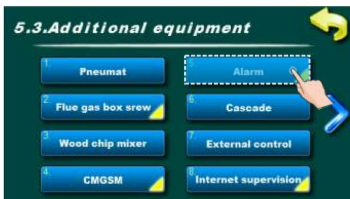
Option for alarm turning ON/OFF (if is installed and configured).
