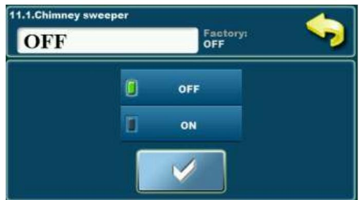
This option allows the flue gas measurement at different boiler powers. When this option is turned on, counter will appear on display. Time will start counting when the boiler reaches selected power (Dx). Text of the counter is red. When the boiler reach the selected power (Dx) and is on selected power for set time and factory set temperature of the boiler is achieved counter turns green and flue gases can be measured.
