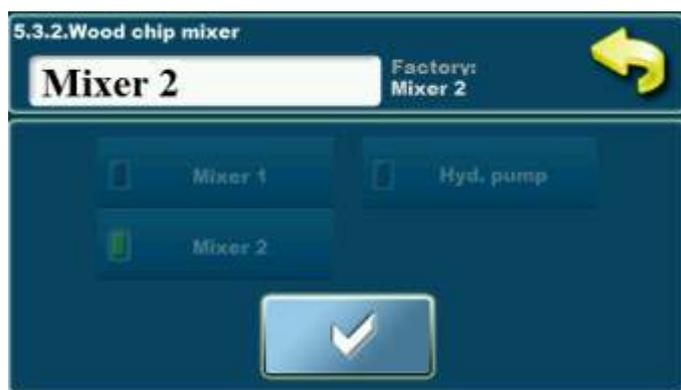
Option for wood chip mixer turning ON/OFF (if is installed and configured). It is not possible to change this parameter.
