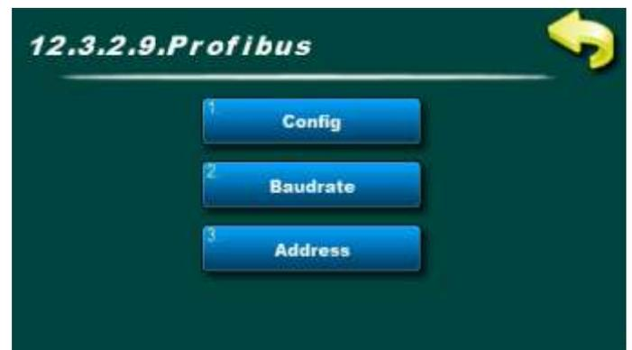
Possibility of configuring the Profibus module (additional equipment). This option can only be configured under a **PIN (authorized service only)**. It cannot be turned ON at the same time as Internet supervision.
