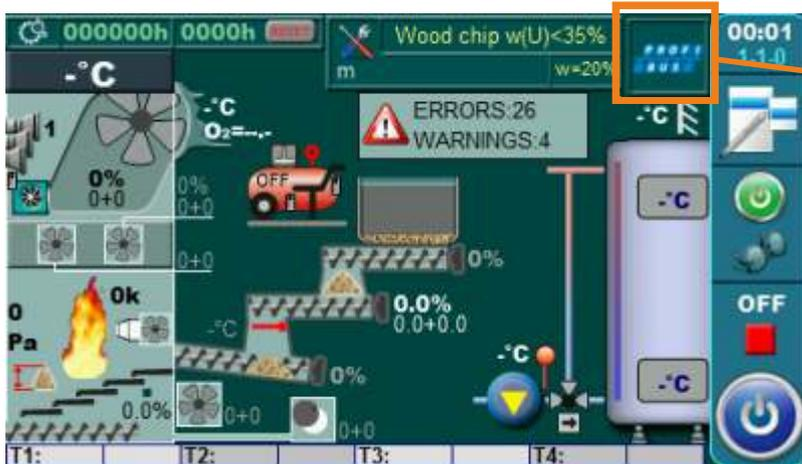
Profibus is configured (selected) in boiler control unit.
