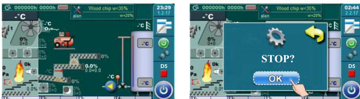
**BOILER IGNITION (boiler start) / BOILER SHUTDOWN (boiler stop) using Schedule**
