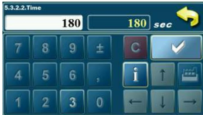
Option for Flue gas box screw turning ON/OFF and adjustment time (if is installed and configured). It is not possible to change this parameter.
