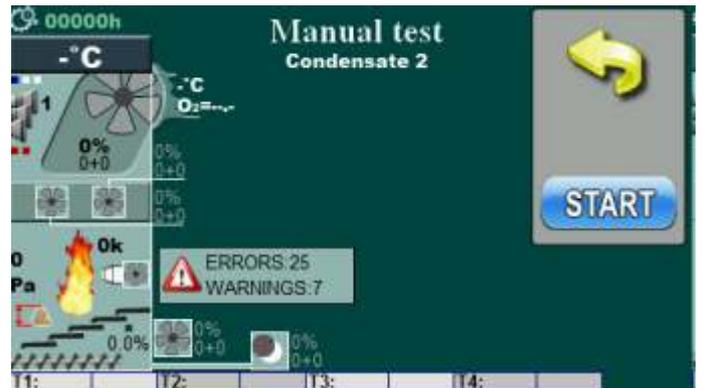
Option for test condensate drainage valve. By pressing „START” button valve will be opened.
