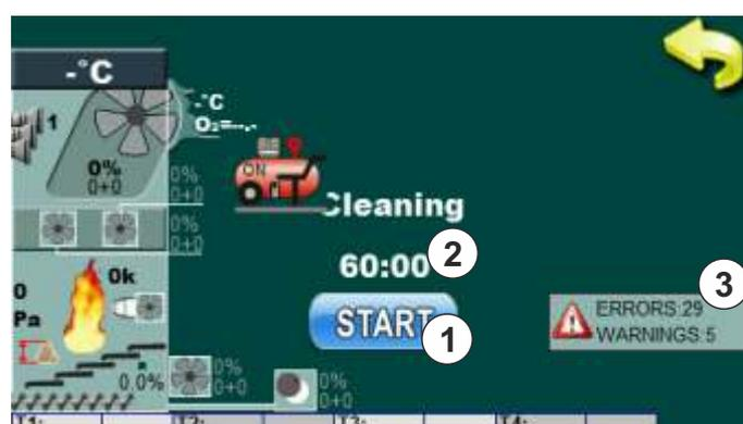
Before cleaning is necessary to start „Cleaning” option by pressing „START” button (1). Depending about which components are selected in point „1.1.3. Type” these components will be start with work with duration of 60 minutes (2). Now is possible to start with cleaning.
