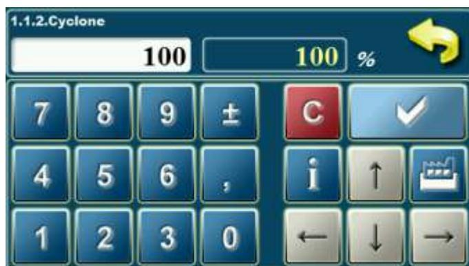
In this parameter is possible to adjust percentage of cyclone work in cleaning option (if is cyclone selected in point „1.1.3. Type”).
