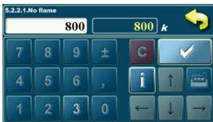
Value of photocell resistance in which will be control unit register that in boiler is no flame. It is not possible to change this parameter.
