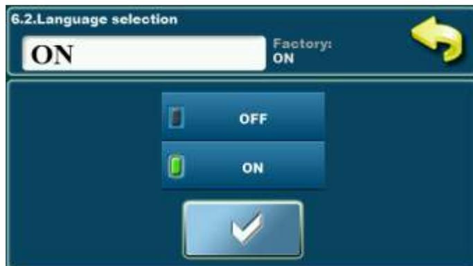
This option enables or disables screen with the choice of language regulation when you turn on main switch. If is marked "OFF", after turning-on the main switch, it will be set on before selected language and after some time, display will show the work display of the boiler.
