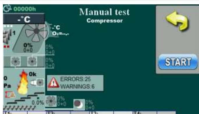
Option for compressor test. By pressing „START” button compressor will be start with work.
