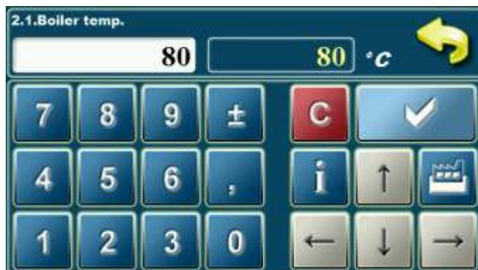
In this parameter is possible to adjust boiler temperature.
