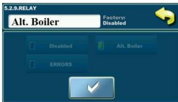
Option for choosing which device will be connected to output relay (alternative boiler or alarm).
