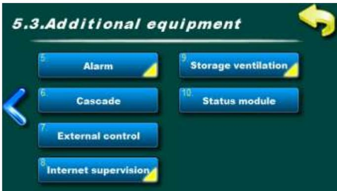
Submenus in this menu depend about installed and configured additional equipment. All installed additional equipment will be showned in this menu (except Profibus and Ash transport).
