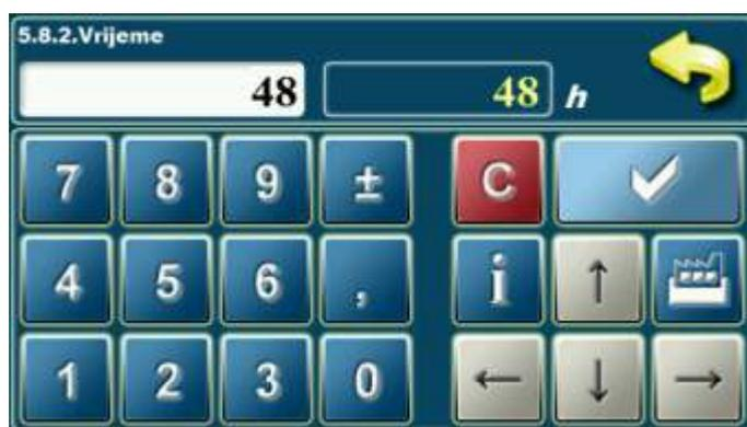
By activating the "Pump protection" option, the setting of the maximum idle time of the output according to the pumps / valves can be adjusted. Factory this option is enabled and max. stand-still time of outputs is set to 48 hours. According to this setting, any pump/valve output that is not activated in 48 hour, it will be activated for a short time.
