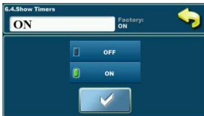
Option for tuning on / off for working hours counter on main screen.
