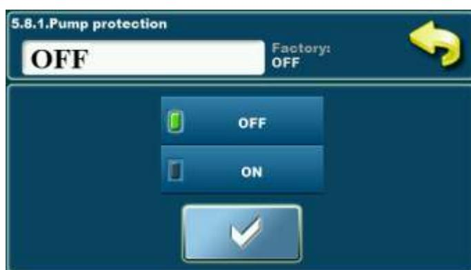
This option enables protection of the pumps/valves from blocking during long stand-still (usually during summer season when heating is off).
