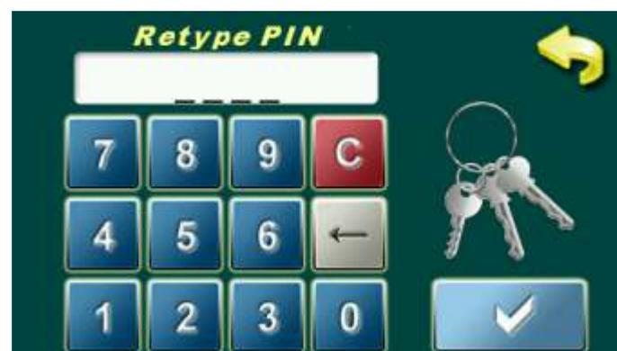
Option for adding new locking user. It's necessary to enter name of user through numerical part (1) and confirm it by pressing confirm button (2). Enter PIN and confirm it. After that is necessary to re-entry PIN and confirm it.
