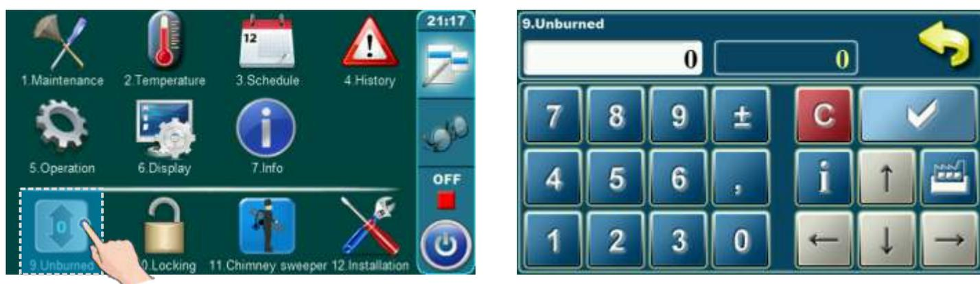
If it appears a lot of unburned fuel in ash box than is possible to use this option which is used for better (completed) fuel burning. With increase value of parameter fuel will be better burn.
