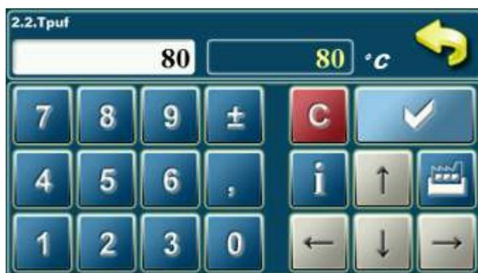
In this parameter is possible to adjust accumulation tank temperature.
