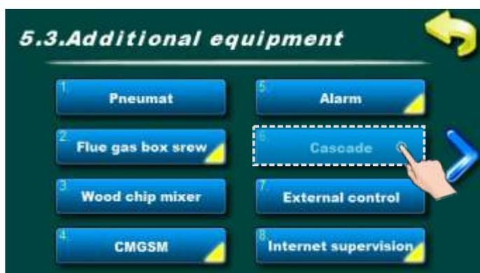
Option for Cascade turning ON/OFF (if is cascade manager installed and configured).
