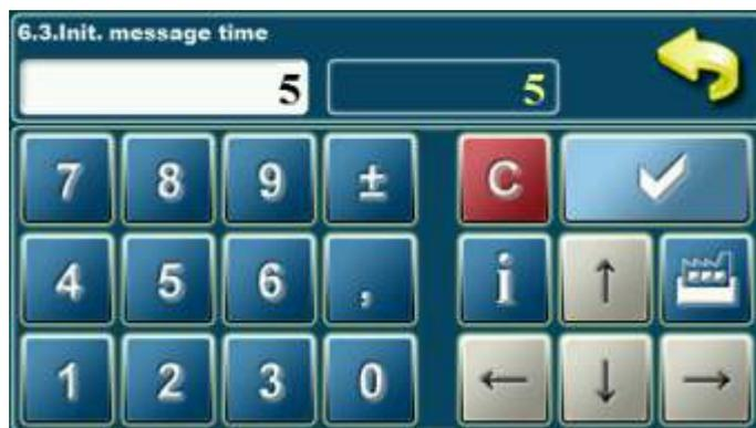
This option is used to set the desired duration of the initial message after turning on the main switch. This option is only available if the option" LANGUAGE SELECTION" (point 6.2.) Is set to"DISABLE".
