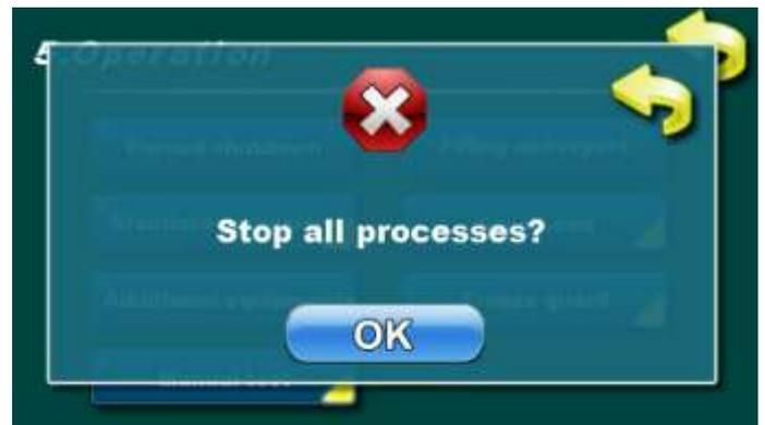
Option for boiler force shut down. By pressing on „OK” button boiler and all boiler processes will be forced shut down.
