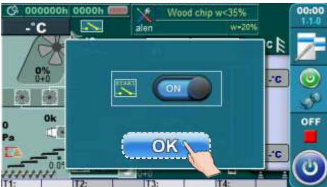
2. Press the ON/OFF button
