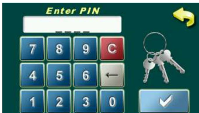
„Installation” menu can be access only with PIN. Only authorized persons have acces pin.”Installation” menu is used by authorized persons for adjustment parameters for boiler work. User can’t access „Installation” menu.
