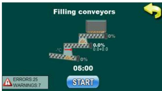
Option for filling conveyors. At start-up or losing fuel, when conveyors are empty then is necessary to use this option for fill them. By pressing „START” button conveyors will be start with work. Use this option until fuel start dropping from conveyors.
