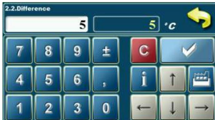
In this parameter is possible to adjust boiler temperature difference.
