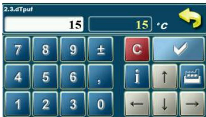
In this parameter is possible to adjust accumulation tank temperature difference.
