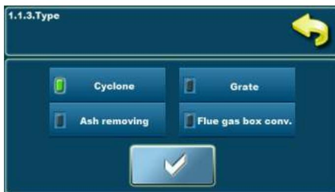
In this parameter is possible to select component which will be work in cleaning option (1.1.1. Cleaning).
