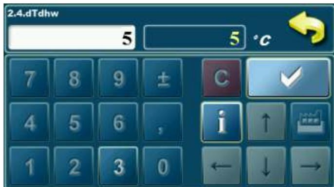
This parameter can't be adjusted. Factory adjusted difference for domestic hot water is 5°C.
