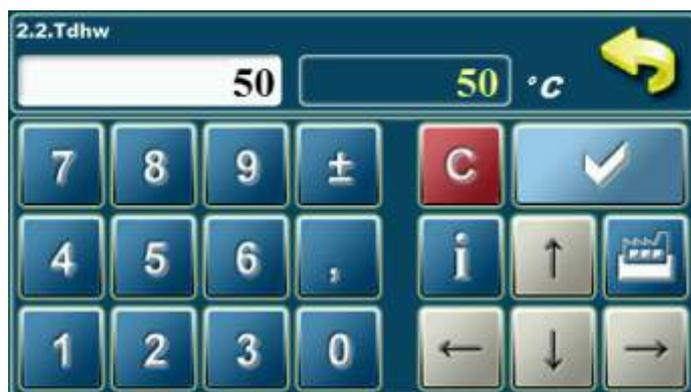
In this parameter is possible to adjust domestic hot water temperature.
