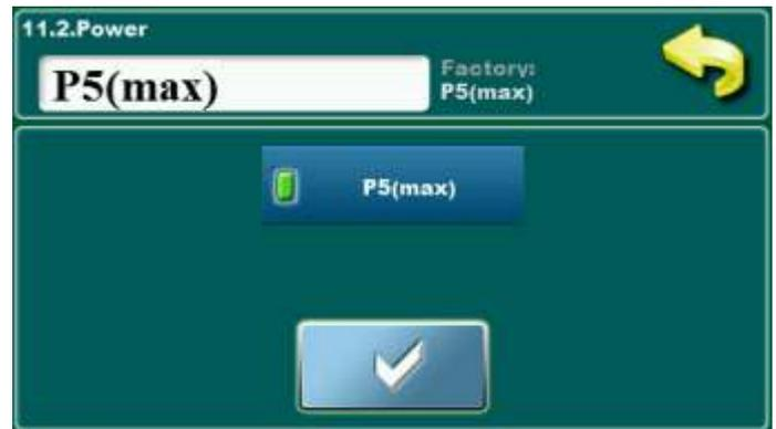
This option allows the boiler to work in different powers in order to measure the flue gases in the boiler modulation phases.
