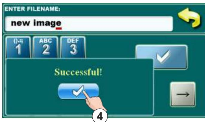
For saving in new image is necessary to press twice on button (1). On display will be displayed option for image name entry. Is necessary to enter image name through numerical part (2). To confirm name press button (3). On display will be displayed message „Successful” which mean that settings are successful saved. Confirm message by pressing button (4).
