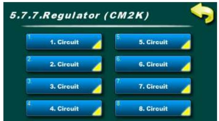
In this menu is possible to change parameters for heating circuits. Number of heating circuits depend about number of installed CM2K modules.
