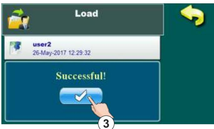
For loading is necessary choose image which we want to load and press on it (1). On display will be displayed message „Are you sure?“. Is necessary to confirm message (2). On display will be displayed message „Successful“ which mean that settings are successful loaded. Confirm message by pressing button (3).
