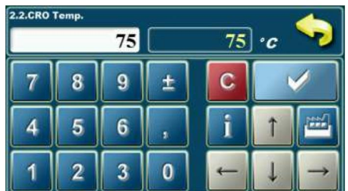
In this parameter is possible to adjust hydraulic crossover temperature.
