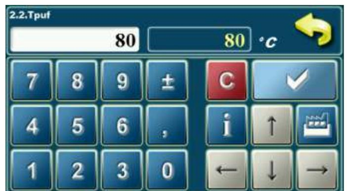
In this parameter is possible to adjust accumulation tank temperature.
