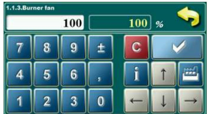
In this parameter is possible to adjust percentage of burner fan work in cleaning option (if is burner fan selected in point „1.1.4. Type”).
