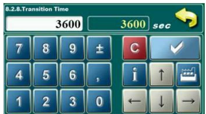
This parameter is used only when configuration doesn't contain room corrector, because regulation doesn't have information of room temperature.
