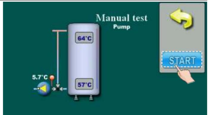
This options enables check of the work for pump between boiler and buffer tank.
