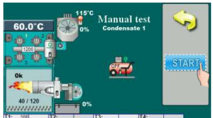
This option allows you to check work of valve for condensate drainage 1. By pressing „START” valve will be opened.
