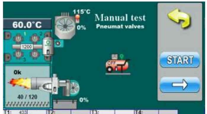
This option allows you to check work of pneumat valves.
