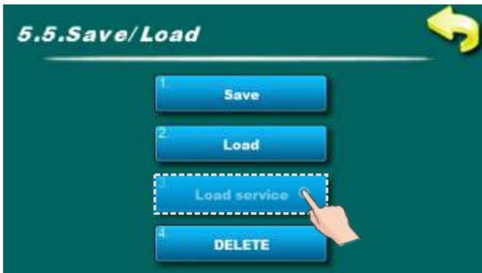
If is needed, with this option i always possible to load setting which is serviceman adjust and saved at first start-up.
