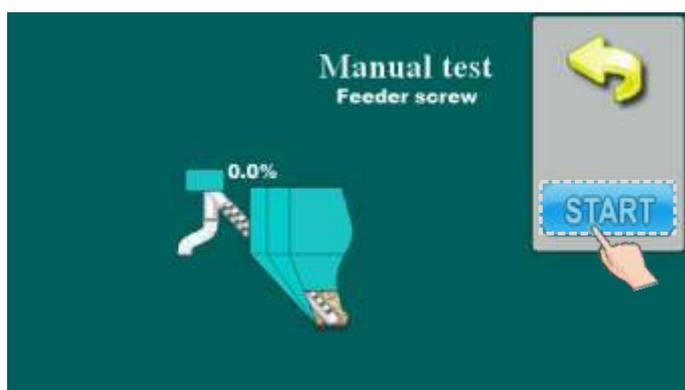
This option allows you to check the motor device of feeding screw.
