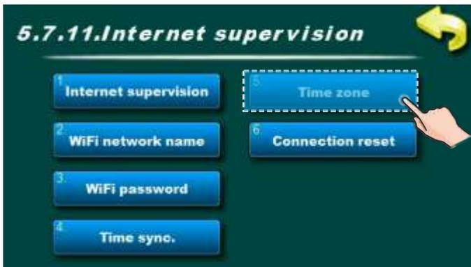
This option allows you to set the time zone if the boiler is in a different time zone than the web portal server. (this option must be set if you enable "Time synchronisation option")
