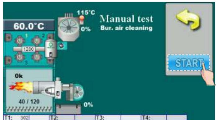
This option allows you to check burner air cleaning work.
