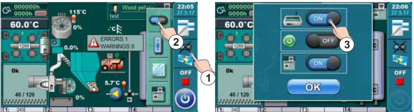
By pressing button for boiler operation (1) on display will be displayed dropdown menu. By pressing button for additional equipment managment (2) on display will be displayed menu for additional equipment managment where is possible to turn on / off additional equipment. Additional equipment menu depend about installed and configurated additional equipment.
