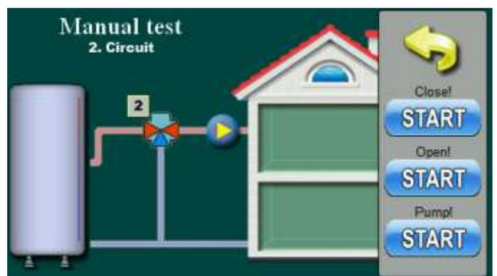
This option allows you to check work pump and mixing valve on 2. heating circuit.
