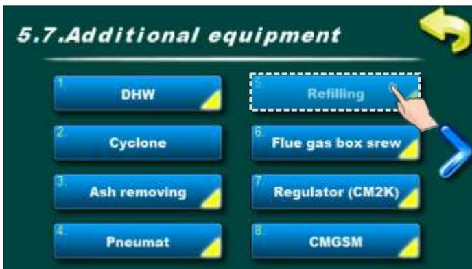
**REFILLING** - refilling the pellet tank (with boiler) from the seasonal pellet tank.
