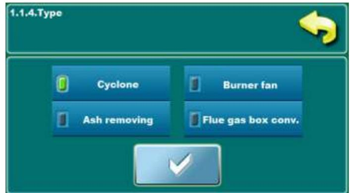
In this parameter is possible to select component which will be work in cleaning option (1.1.1. Cleaning).
