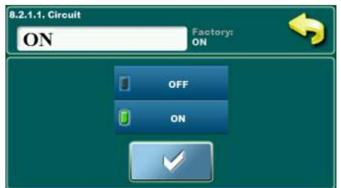
Option for turning on / off first heating circuit.
