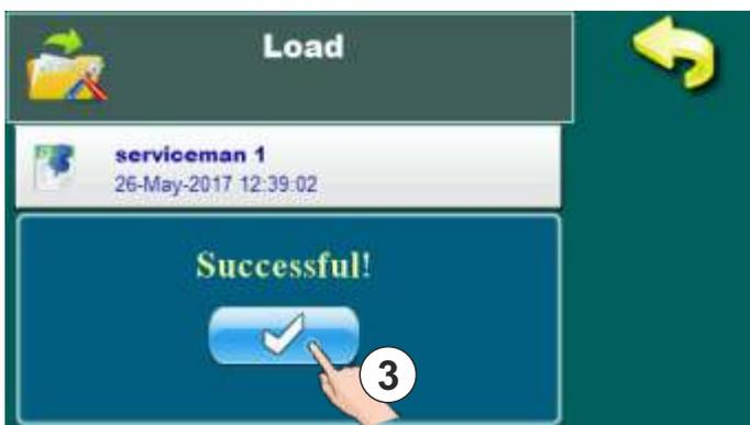
For loading of serviceman settings is necessary to choose image which we want to load and press on it (1). On display will be displayed message „Are you sure?“. Is necessary to confirm message (2). On display will be displayed message „Successful“ which mean that settings are successful loaded. Confirm message by pressing button (3).
