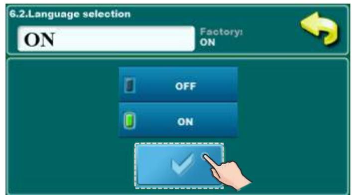
This option enables or disables screen with the choice of language regulation when you turn on main switch. If is marked "DISABLED", after turning-on the main switch, it will be set on before selected language and after some time, display will show the work display of the boiler.(The time until this screen appears can be adjusted in point 6.3.)
