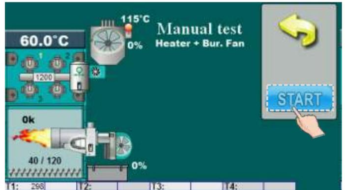
This option allows you to check electric heater and burner fan.
