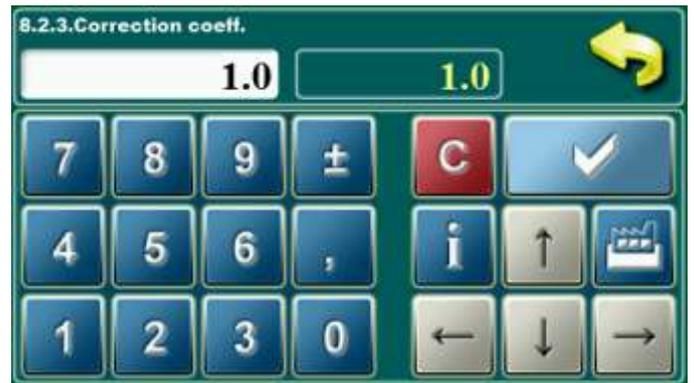
This parameter determines the influence of the room corrector. When this coefficient is larger, room corrector will more affect to the calculated required flow temperature in the heating circuit.
