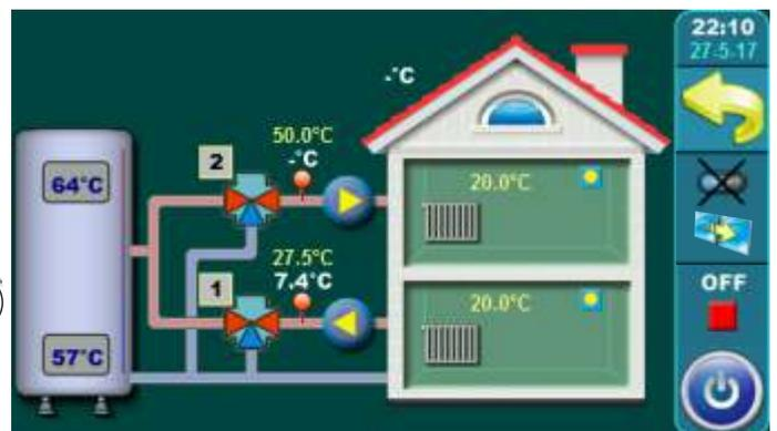
By pressing button for boiler operation (1) on display will be displayed dropdown menu. By pressing button for regulator (2) on display will be displayed heating circuit preview.
