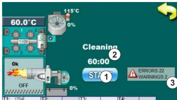
Before cleaning is necessary to start „Cleaning” option by pressing „START” button (1). Depending about which components are selected in point „1.1.4. Type” these components will be start with work with duration of 60 minutes (2). Now is possible to start with cleaning. Pay attention to errors and warnings if they are displayed on the screen (3).
