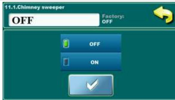
This option allows the flue gas measurement at different boiler powers. When this option is turned on, counter will appear on display. Time will start counting when the boiler reaches selected power (Dx). Text of the counter is red. When the boiler reach the selected power (Dx) and is on selected power for set time and factory set temperature of the boiler is achieved counter turns green and flue gases can be measured.
