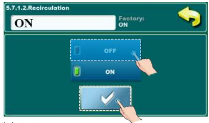
This option allow turning on / off recirculation of domestic hot water.
