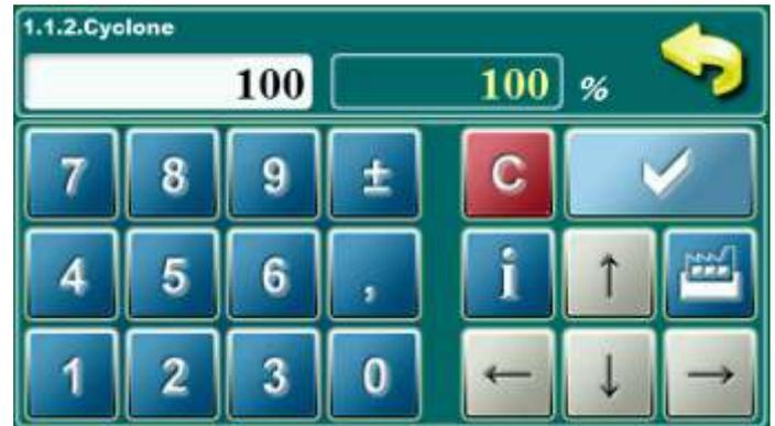
In this parameter is possible to adjust percentage of cyclone work in cleaning option (if is cyclone selected in point „1.1.4. Type”).
