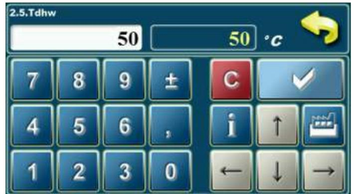
In this parameter is possible to adjust domestic hot water temperature.
