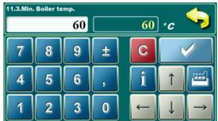
Adjustment of minimal boiler temperature when is chimney sweeper mod activated.
