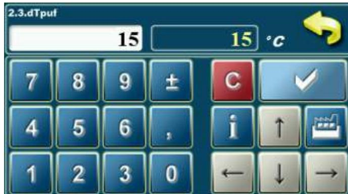
In this parameter is possible to adjust buffer tank temperature difference.
