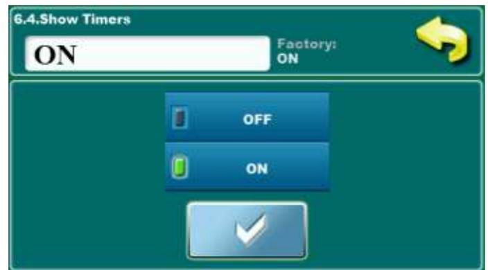
Option for tuning on/off for working hours counter on main screen.
