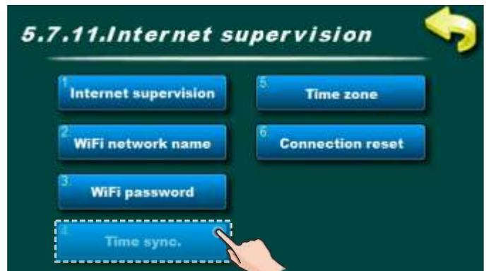
This option allows boiler time synchronization with web server time (internet time).
