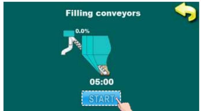
This option allow filling of empty feeder screw with pellets. At start-up or missing fuel, when is feedery screw empty this option is used for filling feeder screw. By pressing „START” feeder screw start with work. This option must be turned on until fuel start dropping from feeder screw.
