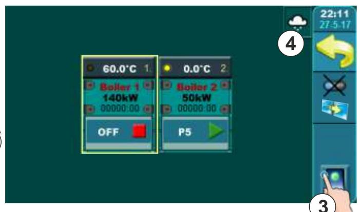
By pressing button for boiler operation (1) on display will be displayed dropdown menu. By pressing button for cascade management (2) on display will be displayed menu for cascade management. By pressing button (3) is possible to start / stop boiler in cascade. On toolbar (4) are shown which of SUMMER / WINTER mode is active.
