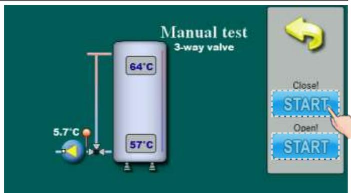
This option allows you to check the work for 3-way mixing valve.
