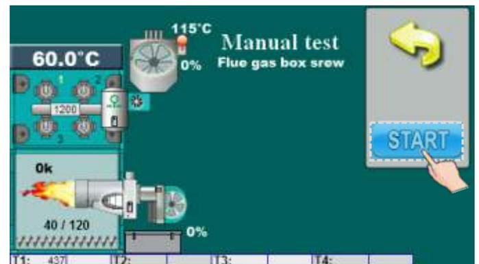
This option allows you to check work of flue gas box cleaning system.
