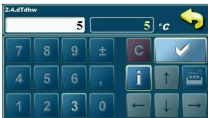
This parameter can't be adjusted. Factory adjusted difference for domestic hot water is 5°C.
