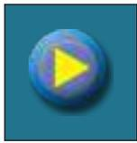
Pump (when pump is working symbol is rotating, otherwise idle)
