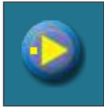
The pump has a request for work (next to the pump symbol bright yellow square when the consumer given the demand for work the pump, the pump does not work if you have not met all the conditions for work, for example. low temp. in the boiler, otherwise the pump normally works)
