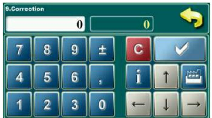
If it appears a lot of unburned fuel in ash box than is possible to use this option which is used for better (completed) fuel burning. With increase value of parameter fuel will be better burn.
