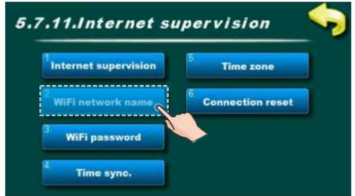
This option allows you to enter the name of WiFi home network to which you want to connect the "Cm WiFi box" and the boiler. You must enter exact WiFi network name or else boiler will not be able to connect to the WiFi network.
