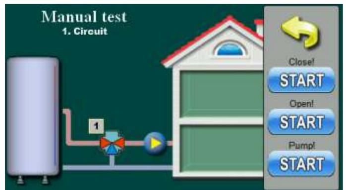
This option allows you to check work pump and mixing valve on 1. heating circuit.
