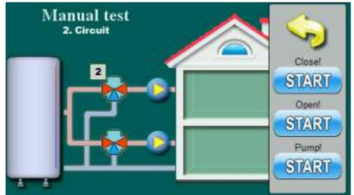
Option for testing elements of 1st heating circuit (mixing valve (START-open), mixing valve (START-close) and pump (START)).
