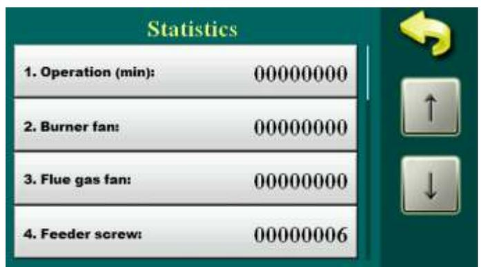
The regulation follows the startup number of the boiler and the work time of certain parts of the boiler.
