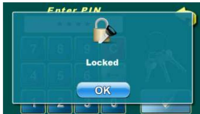
Option for locking display. Display can be locked only if exist profile for locking (10.2. Add user; 10.4. User list). When is display locked is possible to move through all menus but parameters can't be changed.
