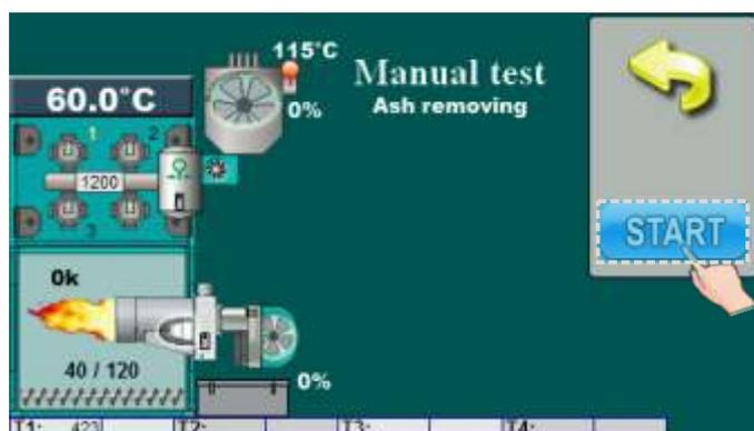
This option allows you to check work of ash removing by conveyor.
