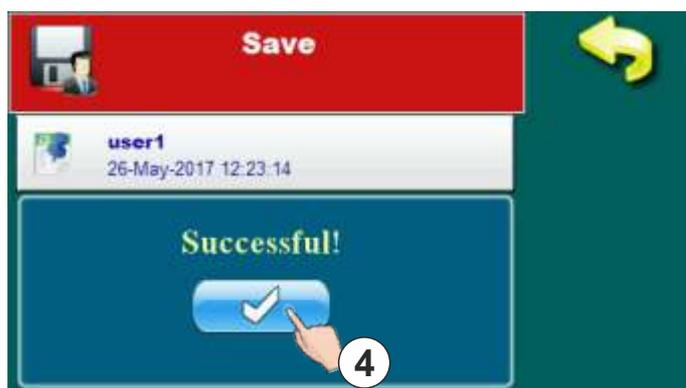
For saving in existing image is necessary to press on exist image (1). On display will be displayed message „Are you sure?”. Is necessary to confirm message (2) and press button for saving confirmation (3). On display will be displayed message „Successful” which mean that settings are successful saved. Confirm message by pressing button (4).
