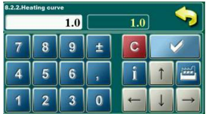
This parameter determine the coefficient of the heating curve. The regulation calculate required flow temperature according to the heating curve and outside temperature to achieve the desired room temperature.
