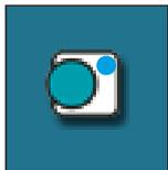
Next to the room thermostat symbol bright blue circle (the room thermostat has requested for operating the pump, the pump does not work if you have not met all the conditions for its operation, for example. low temp. in the boiler, otherwise normally works)
