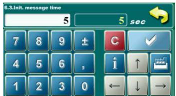
This option is used to set the desired duration of the initial message after turning on the main switch. This option is only available if the option" LANGUAGE SELECTION" (point 6.2.) Is set to"DISABLED".
