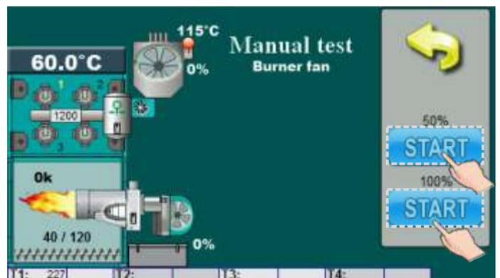
START 50% - fan speed must be on 50%
