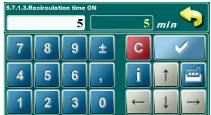
In this parameter is possible to adjust working time for recirculation.
