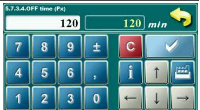
In this parameter is possible to adjust ash removing off time.
