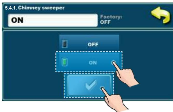
When this option is turned ON, button "BOILER OPERATION DISPLAY" becomes a button "CHIMNEY SWEEPER" (1). Pressing this button directly opens the menu "CHIMNEY SWEEPER" (without the need for scrolling through the menus). In this menu, is access to change parameters of "CHIMNEY SWEEPER" menu.
